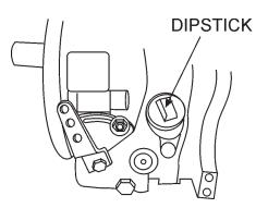
Figure 5. Engine Oil Dipstick (Removal)
